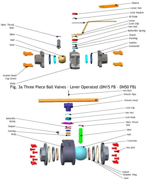
Fig. 3b Three Piece Ball Valves - Wrench Operated (DN65 FB - DN100 FB)
