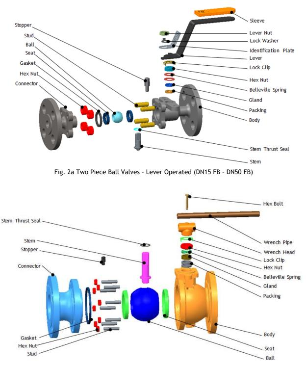
Fig. 2b Two Piece Ball Valves - Wrench Operated (DN65 FB - DN150 FB)
