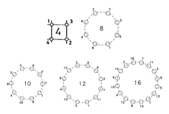
Fig. 7 Tightening Sequence
