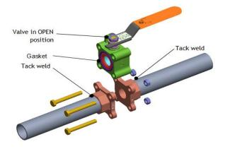
Fig. 5 Three-piece ball valves Welding
